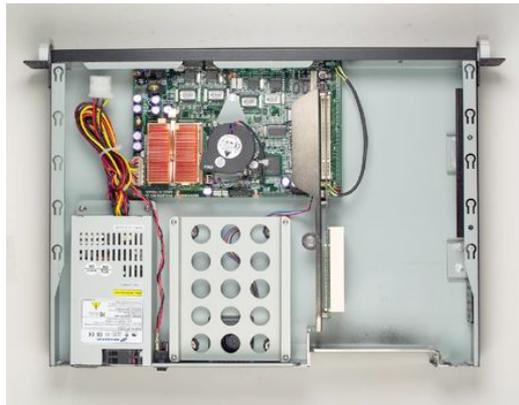
**Figure 5-1: Reference Design to be used in IST2004**
